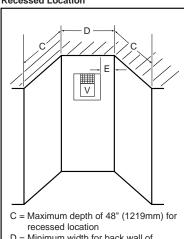
D = Minimum width for back wall of recessed location -Combustible - 38" (965mm)
